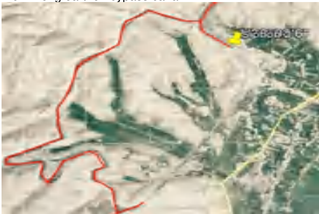
Photo 9. Non-functional Loikasoi Siphon (No. 2) comprising two Steel pipes 590 m long at 38°8'01"N, 68°49'54"E, and the 4.1 km long bypass canal. Lining required.
